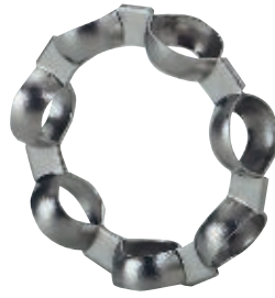
myonic cage "48" Two piece steel ribbon cage loosely crimped for low torque
